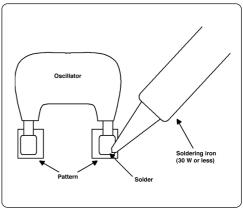
Figure 3.5 Removing an oscillator
